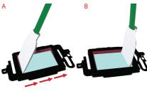
Both sides of the swab may be used to clean. Use each side of the swab only once during cleaning. Cleaning with a contaminated swab edge can potentially harm the sensor. You may be required to add additional cleaning solution to the opposite side.
