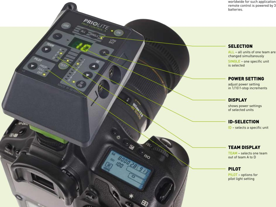
All Priolite flash units and the LED 400 work perfectly together with the Priolite remote control units, which are attached to the hot shoe of the camera. Almost all functions of the flash unit can be controlled remo-
