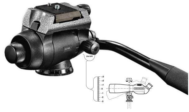
The G2180 has an accurate and fully adjustable counterbalance system. The system can be engaged or disengaged, and has 7 pre-set positions to help it balance up to 2.5kg/5.5lbs offset weight. For more precise balance control we suggest the use of a long quick release plate.
