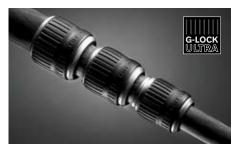
New Mountaineer tripods feature G-lock Ultra, a redesigned version of Gitzo's signature leg lock system G-lock. G-lock Ultra has even more comfortable operation and reduced risk of debris entering the tubes and locking mechanisms. It is fine-tuned for the smaller differences in tube diameter between leg sections of Carbon eXact tubes, contributing to increased stiffness of the legs.
