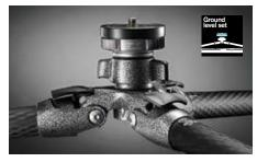
The Ground Level Set mechanism, which lets the photographer remove the centre column to get the camera closer to the ground, has been completely redesigned for faster operation. A single simple unlocking ring under the column's upper disc frees the column while keeping the upper disc solidly in place on the tripod, with no need to unscrew and re-fit the upper disc and hook as in previous versions.
