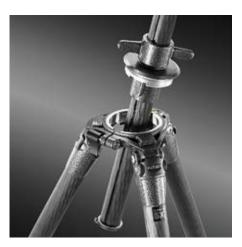
A Systematic tripod allows a choice between various centre columns, flat plates, video half-bowls and accessories. Most Systematic tripods are supplied with a flat plate, but the optional Systematic accessories can be fitted by simply unlocking the lever in the top casting, lifting out the flat plate and fitting in the alternative accessory.
