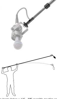
Gitzo booms feature a 1/4" - 3/8" reversible mounting screw supported by a high quality machined aluminium upper end. The microphone cable can be run either outside or inside the pole. The aluminium upper end is specially provided with a machined hole for inner cables.
