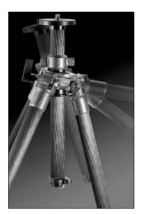
The centre column can be inclined in any direction at any angle up to 15°. Leg angles can be set independently at any of the three positions. A leveling tripod is an ideal support for fluid heads, setting the camera perfectly horizontal while allowing the fluid head to control pan and tilt movements.
